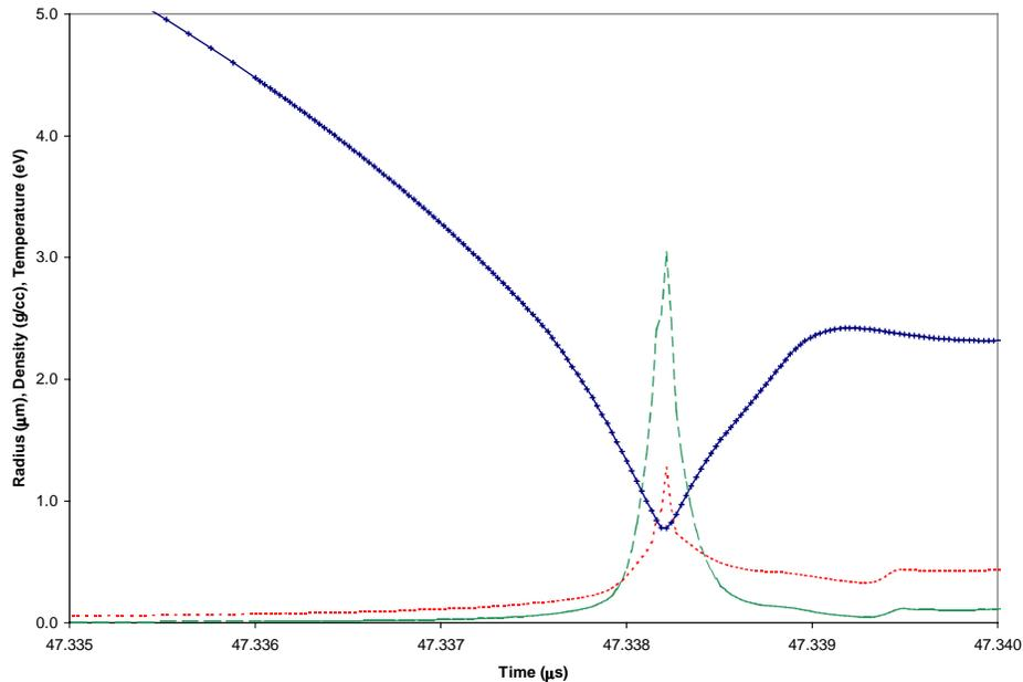
Figure 14. Bubble radius (solid line with dots at the plotting times), and typical bubble density (long-dashed line) and temperature (short-dashed line) histories near the bubble’s collapse time. In this calculation, without thermal conduction effects, the peak temperature and pressure occur near-simultaneously with the peak gas density and minimum bubble radius. The density history shown here is used to estimate the duration of the radiation pulse emitted upon bubble collapse.
