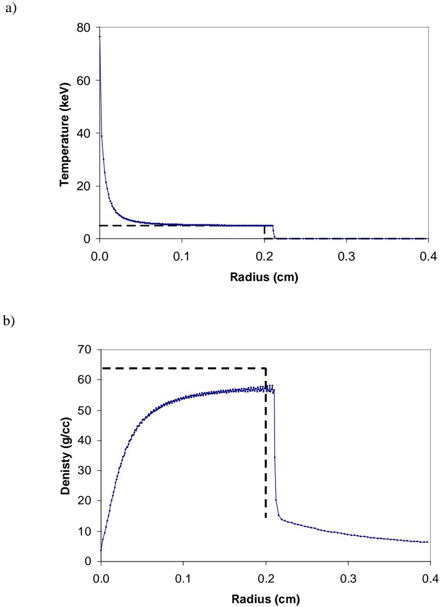
Figure 3. Noh problem (a) temperature and (b) density as calculated by HYADES (smooth curve with dot plotted for each zone-center value) and expected from analytic solution (dashed lines). Like many hydrodynamics codes, HYADES generates spurious heating in the zones near the singularity at the origin.
