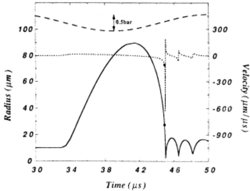
Figure 6. Reprinted from ref. 2, figure 1. Moss's Step 1 calculated history of the bubble interface radius (solid curve) and velocity (short-dashed curve). The long-dashed curve is the oscillatory driving pressure, retarded by the sound transit time into the vicinity of the bubble.
