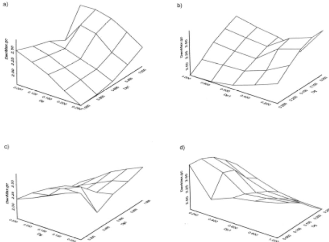
Figure 12. Maximum gas density at the center of the bubble behaves much more non-linearly as the mesh is refined. One significant factor in this behavior is the development of a strong shock in the finer-zoned runs, as shown in Fig. 10. Even in this case, as the mesh is refined, the convergence appears to be approaching a linear regime.
