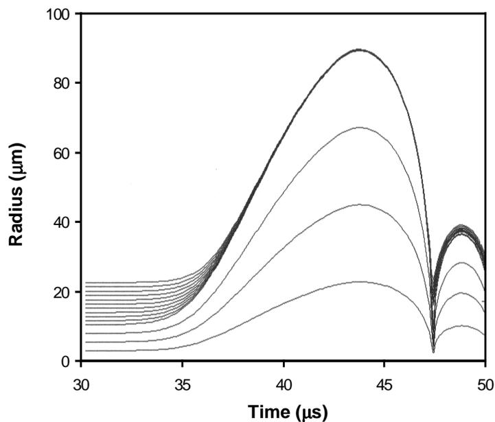
Figure 7. Radius history for the four air zones and the innermost 10 water zones in the first HYADES simulation of the SL test case. Compare this result with that of Moss, et al. in Figure 6. Qualitative and semi-quantitative agreement is readily seen.
