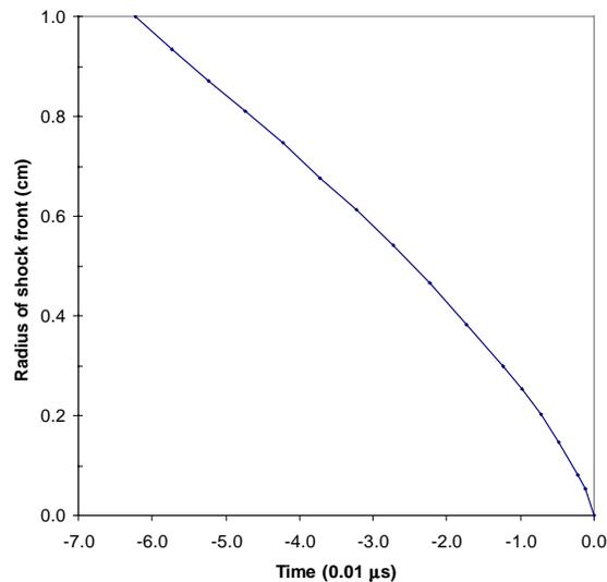
Figure 5. Radius history of the inward-moving shock front in the Guderley simulation. Plotted points were extracted by hand from the HYADES simulation at selected times. The abscissa is the time before the shock reaches the origin (as used in the similarity solution), in units of  $0.01 \mu\text{s}$ . From this curve, we extract the similarity solution's parameter,  $\alpha = 0.75 \pm 0.03$ , in reasonable agreement with the results of Stanyukovich's numerical solution [ref. 13, p. 803].
