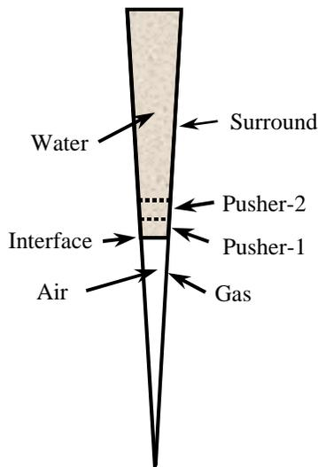
Figure 8. Schematic diagram of the physical regions considered for the zoning and convergence study. Drawing is a pie-diagram representation of a segment of the sphere, and is not to scale.
