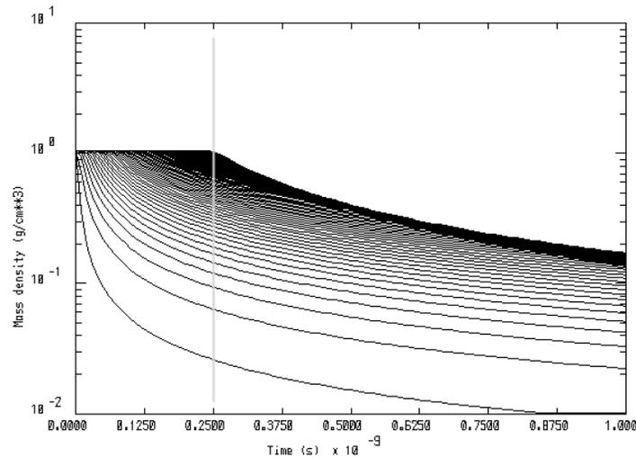
Figure 1. History of the mass density of every zone in the planar expansion test problem shows the successive density decreases as the rarefaction wave develops. The gray solid line shows the time the rarefaction is expected to reach the center of the foil. HYADES reproduces expected features of the expansion quite well.
