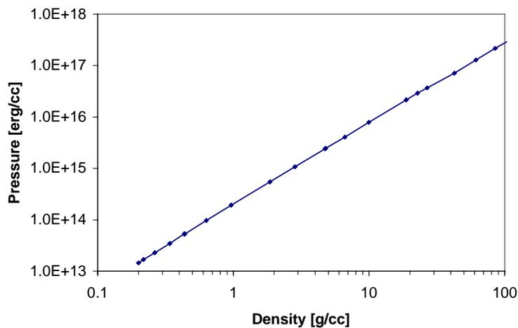
Figure 2. Isentropes of a single zone in the planar isentropic compression test case. Using an ideal gas equation of state, HYADES (dots) matches the expected isentropes (solid line) for  $\gamma = 5/3$  to better than 5%.
